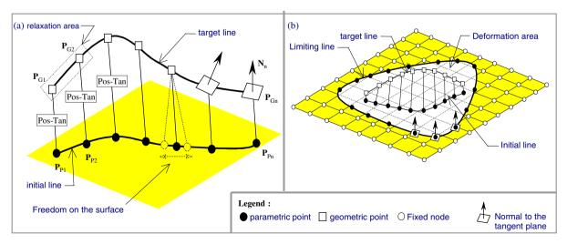
Fig. 7. Target (a) and limiting (b) line specification.
