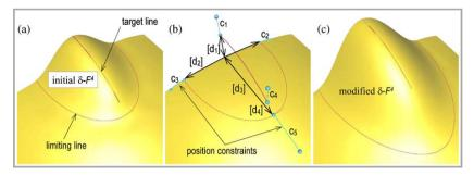
Fig. 14. Modifications of numerical parameters defining a  $\delta$ -F<sup>4</sup>: increase of the length ( $d_3$ ), the heights ( $d_1$  and  $d_4$ ) and the depth ( $d_2$ ).
