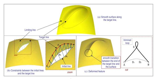
Fig. 9. Insertion of  $G^1$  discontinuity along the target line.
