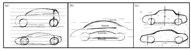
Fig. 1. (a) Character lines in a car. (b) Volumes of different cars. (c) Symmetry vs. asymmetry of the roof line.
