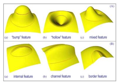
Fig. 6.  $\delta$ -F<sup>4</sup> shape characterisation according to morphological (A) and topological (B) criteria.
