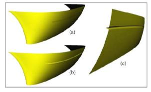
Fig. 13. Shape modification by direct instantiation of character lines, applied to a car rear bumper.
