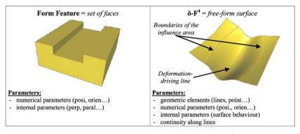
Fig. 4. Comparison between form features and  $\delta$ -F<sup>4</sup>.
