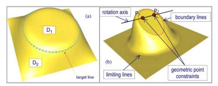
Fig. 11. (a) Planar area obtained by minimisation. (b) Planar area obtained by constraints (only a line of the final plane is prescribed).
