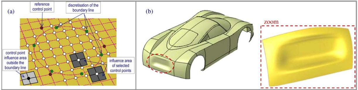
Fig. 12. (a) Co-planarity constraints on selected nodes and on points of the boundary line, with 3 nodes as references. (b) Insertion of a planar surface for the number plate of a car (courtesy of *Pininfarina Ricerca e Sviluppo*).
