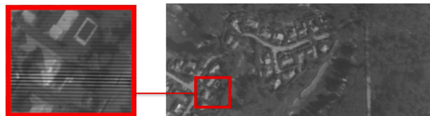
Fig. 1. An image from Sieleters. On the left, a magnified detail shows contrasted interference fringes.
