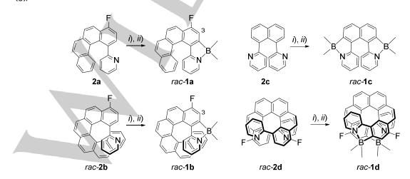
Scheme 2. Synthetic routes to azabora[n]helicenes 1a-d. i) BBr<sub>3</sub>, N<sup>i</sup>Pr(Et)<sub>2</sub>, CH<sub>2</sub>Cl<sub>2</sub>, 25°C, 24 hrs; ii) AIMe<sub>3</sub>, CH<sub>2</sub>Cl<sub>2</sub>, 30 min.
