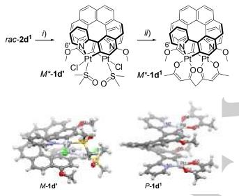
**Scheme 4.** Synthesis and X-ray structures of bis-platina[10]helicenes **1d'** and **1d<sup>1.§</sup>** *i*) Pt(dmso)<sub>2</sub>Cl<sub>2</sub>, Na<sub>2</sub>CO<sub>3</sub>, toluene, reflux, 84%; *ii*) acacNa, toluene, reflux, 57%.
