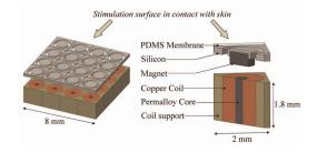
Figure 4: PDMS magnetically actuated [35].
