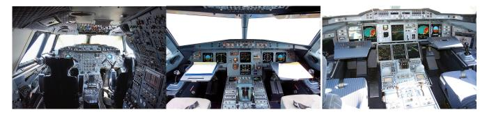
Figure 2: Types of cockpit. Left: Concorde's analog cockpit; Center: glass cockpit in the A320; Right: interactive cockpit in the A380.
