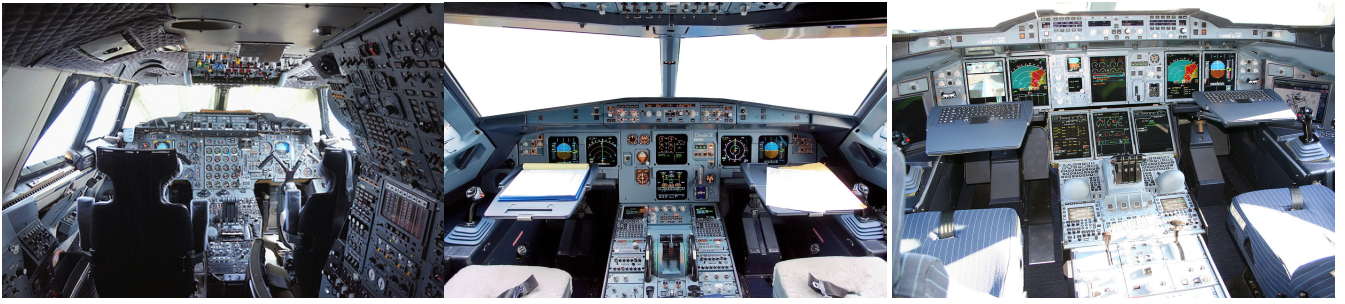
Figure 2: Types of cockpit. Left: Concorde’s analog cockpit; Center: glass cockpit in the A320; Right: interactive cockpit in the A380.
