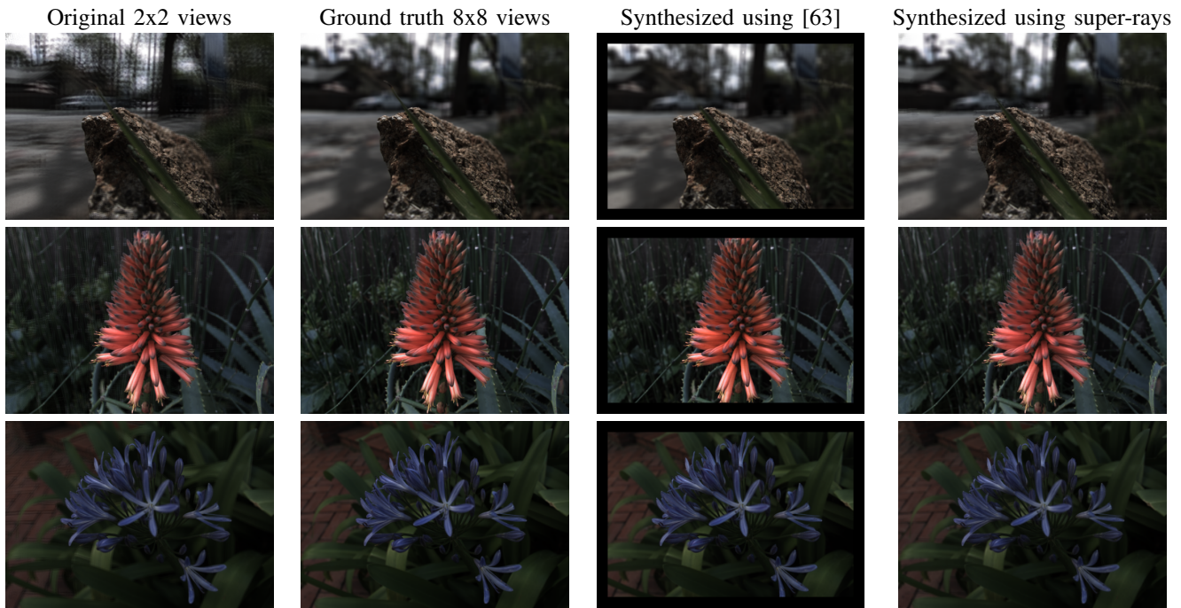
Fig. 11: Angular aliasing comparison. We show the images refocused with the 2x2 corner views in the test set in [63], the full 8x8 light field (ground truth), the 8x8 synthesized light field with the approach in [63] and the 8x8 light field synthesized with our approach. We use k = 1000 and m = 1 .
