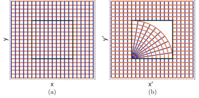
FIG. 8. (Color online) Transformation of the bend from Ref. [18] and used in Sec. IV A for an angle of  $\beta = \pi/2$ . The Cartesian  $x$ - $y$  grid within the quadratic subdomain in panel (a) is transformed in such a way that grid lines of constant  $y$  transform into lines of constant radial coordinate  $\rho'$  in panel (b) and similarly lines of constant  $x$  transform into lines of constant azimuthal coordinate  $\varphi'$ .
