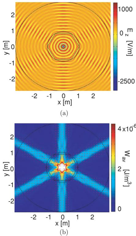
FIG. 4. (Color online) Simulation of an  $N$ -beam directional antenna for  $N = 6$ . Using the refractive index distribution from Fig. 2(b) the cylindrical waves that are emitted from the line source at the origin are transformed to hexagonal wave fronts that finally form the six beams of the antenna. Panel (b) shows the corresponding total energy density.
