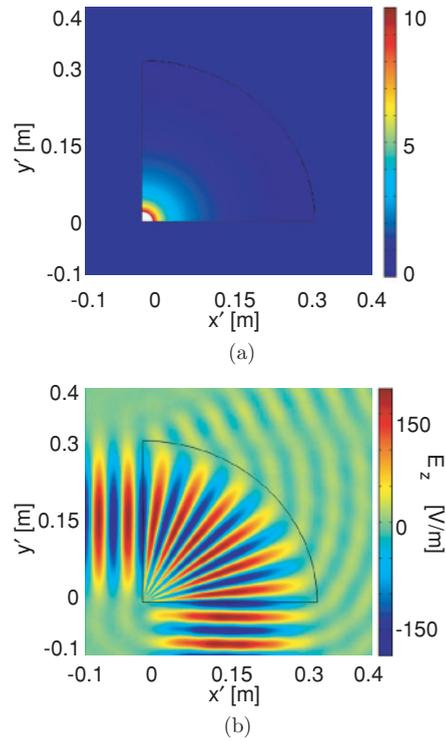
FIG. 9. (Color online) (a) Refractive index distribution for the isotropic perpendicular bend of width  $w = 0.3$  m from Eq. (12) in Sec. IV A. For better visual perception, the shown refractive index is limited to  $n' = 10$ . (b) Propagation of a TE-polarized Gaussian beam at a free space wavelength of  $\lambda_0 = 0.05$  m that impinges from the left on the bend.
