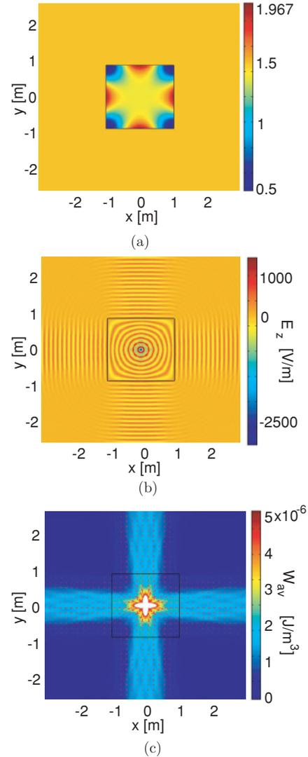
FIG. 3. (Color online) Simulation of the four-beam directional antenna. (a) The refractive index distribution  $n'$  that is used and obtained from the one in Fig. 2(a) by scaling with a factor of 1.5 and restricted to  $n' > 0.5$ . This medium transforms the cylindrical waves emerging from the line source at the origin of panel (b) to quadratic wave fronts that finally form four collimated beams leaving the antenna. Panel (c) shows the corresponding total energy density.
