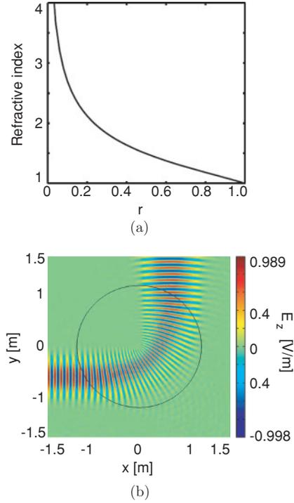
FIG. 12. (Color online) (a) Radial refractive index profile  $n(r)$  for the perpendicular bend according to Eq. (16). While the refractive index diverges for small radii  $\rho = rR$ , it exhibits a continuous transition to the outer space at the interface, that is, for  $r = 1$ . (b) Propagation of a TE-polarized Gaussian beam through a bend with a radius of  $R = 1$  m confirming its functionality.
