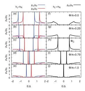
Fig. 4: (Colour online) LDOS of the junction  $\rho(E)$  divided by the normal state LDOS  $\rho_0(E)$ , for parallel (left column) and anti-parallel (right column) orientation of the exchange fields of magnitude  $|h_{\rm L,R}|/\Delta=0.3$ . The phase difference gradually increases from the top panels where  $\phi=0$  through  $\phi_{\rm C}$  to the bottom panels with  $\phi=\pi$ . All plots are for  $\tau=1.0$ .
