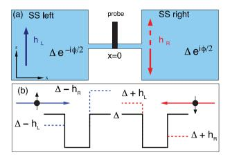
Fig. 1: (Colour online) (a) Schematic diagram of the junction. Two SS electrodes with intrinsic exchange fields  $h_{\rm L}$ ,  $h_{\rm R}$  separated by a ballistic weak link. A tunneling probe is situated at x=0. (b) Sketch of the effective gaps for spin-up/down electron when the left/right exchange fields  $h_{\rm L}/h_{\rm R}$  are configured so that  $-h_{\rm R} > h_{\rm L} > 0$ .
