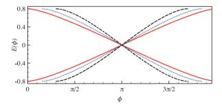
Fig. 3: (Colour online) Discrete part of the spectrum of a SS/N/SS junction as a function of the phase across the junction in the anti-parallel configuration ( $h_{\rm L}=-h_{\rm R}=0.2$ ) for three different lengths of the junction: L=0 (dashed black line),  $L=0.3\xi$  (dotted blue line) and  $L=0.6\xi$  (solid red line).
