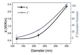
Fig. 1 Plot of the thermal conductivity (black spheres) and the orientation parameter,  $\Gamma$ , (blue stars) of P3HT NWs as a function of the NW diameter.  $\Gamma = \gamma \mu/1.18\gamma_{\parallel}$ , where  $\gamma_{\parallel}$  and  $\gamma_{\parallel}$  are the areas of the (100) peaks in directions perpendicular and parallel to the NW axis, respectively. The coefficient 1.18 is extracted from the ratio  $\gamma_{\parallel}/\gamma_{\parallel}$  of the bulk P3HT.
