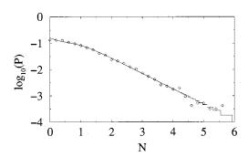
FIG. 5. Probability density P of normal forces in a packing at static equilibrium fitted by the form  $f(N) = a(1 - be^{-N^2})e^{-\beta N}$ , with b = 0.6 and  $\beta = 1.35$ , proposed by Mueth et al. Forces are normalized with respect to the mean force.
