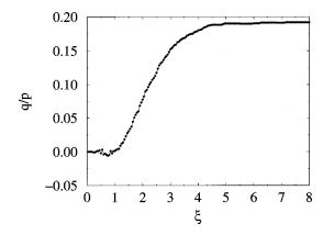
FIG. 9. Contribution of the forces below  $\xi$  to the stress ratio q/p as  $\xi$  is increased from zero to the maximal force in a simple shear simulated by the MD method.
