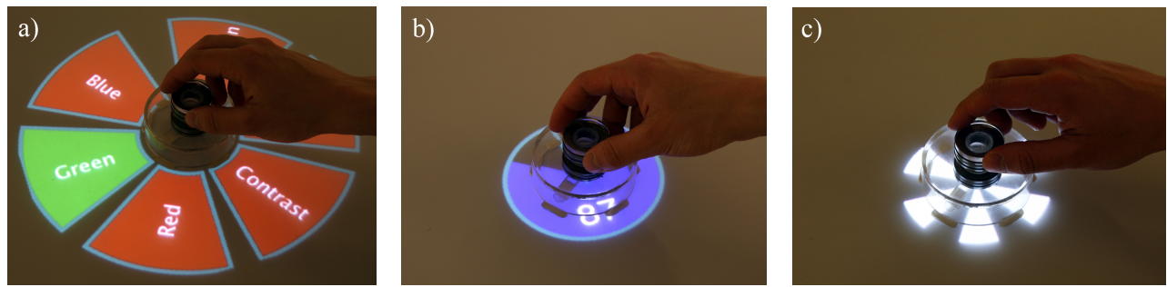
Figure 4. SLAP Knob user interface. a) Selecting image property from menu. b) Setting continuous value. c) Relative navigation for frame stepping in videos.
