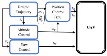
Fig. 5. Octo-Rotor control architecture.
