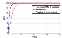
Fig. 6. Response for altitude motion in stationary flight.
