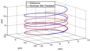
Fig. 12. 3D tracking using Nonlinear IMC-Feedback (Persistent disturbances of 23N).
