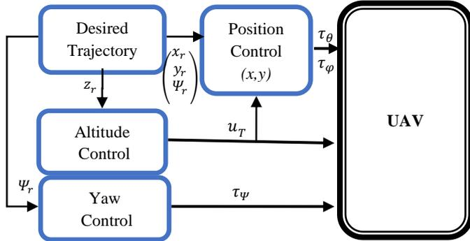
Fig. 5. Octo-Rotor control architecture.
