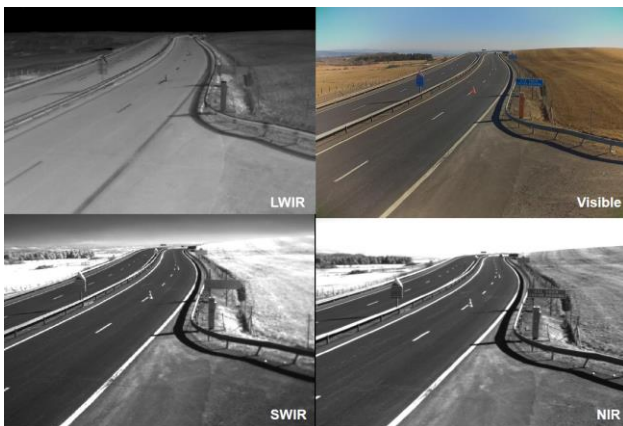
Figure 3: Example of video records by LWIR (top left), Visible (top right), SWIR (bottom left) and NIR (bottom right) cameras
