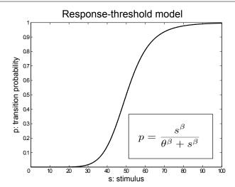
Fig. 2: The response threshold function. The transition probability p depends on: s, a stimulus that represents a measure of the transition urgency;  $\theta$ , a threshold on the stimulus; and  $\beta$ , a sensitivity parameter. The function is non-linear: When  $s \ll \theta$ , the transition probability is very low, whereas when  $s \gg \theta$  it is very high. In the example in the figure, s ranges in [0, 100],  $\theta = 50$  and  $\beta = 8$ .
