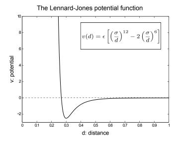
Fig. 3: The Lennard-Jones potential function. The potential v depends on the current distance d between two robots.  $\sigma$  is the desired distance between the robots and  $\epsilon$  corresponds to the depth of the potential function. In this example,  $\sigma=0.3$  and  $\epsilon=2.5$ .
