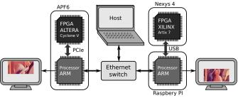
Fig. 2. Experimental setup.
