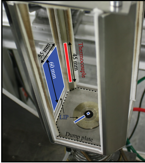
Fig. 2. Photograph of the combustion chamber showing the location of temperature measurements for the characterization of the thermal boundary conditions in the combustor.
