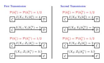
Fig. 3. In both transmissions, the capacity of the channel to the legitimate decoder takes two possible values  $\{4,5\}$  with probability (1/2,1/2) and the capacity of the channel to the eavesdropper takes two possible values  $\{2,3.5\}$  with probability (1/2,1/2).
