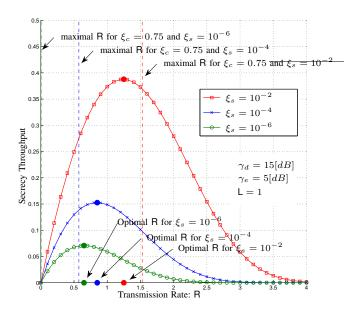
Fig. 8. Secrecy throughput depending on the secrecy rate R  $\geq 0$ , for different secrecy constraints  $\xi_{\rm s} \in \left\{10^{-2},10^{-4},10^{-6}\right\}$  and a single L=1 transmission. Vertical dashed lines represents the maximal secrecy rate R corresponding to the constraint  $\xi_{\rm c}=0.75$ .
