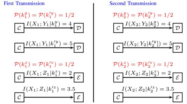
Fig. 3. In both transmissions, the capacity of the channel to the legitimate decoder takes two possible values  $\{4, 5\}$  with probability  $(1/2, 1/2)$  and the capacity of the channel to the eavesdropper takes two possible values  $\{2, 3.5\}$  with probability  $(1/2, 1/2)$ .
