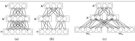
Figure 2: Architectures of deep neural networks: (a) – Deep Boltzmann Machine with 2 hidden layers, (b) – 1D SBM with 2 patches, (c) – 1D MSBM with 2 patches and 2 object parts.
