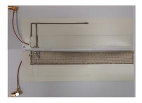
Figure 5. Photography of the ARGOS PIFA textile antenna.
