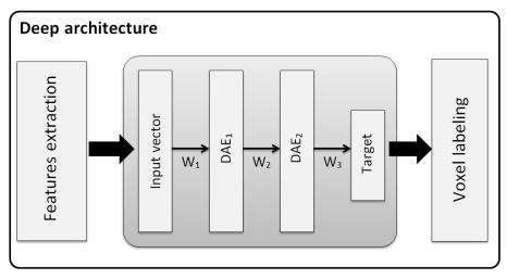
Figure 4: Deep network architecture constructed by stacking denoising autoencoders in the proposed approach.
