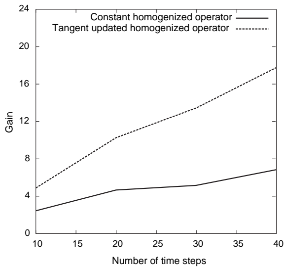
Fig. 11. Evolution of the gain as a function of the number N of time steps.
