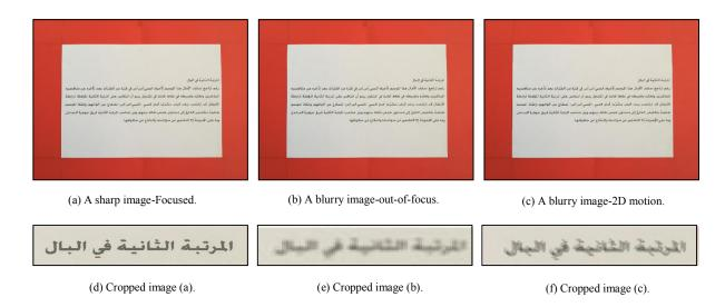
Figure 5. Examples of captured images for single distortions.
