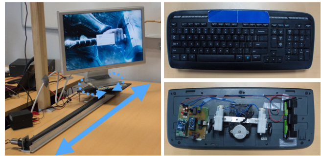
Figure 3. Left. The monitor relies on a servo motor for rotation and a rail for translation. Right. The keyboard is augmented with a robotic base allowing translation ( T_{xz} ) and rotation ( R_y ) of the device
