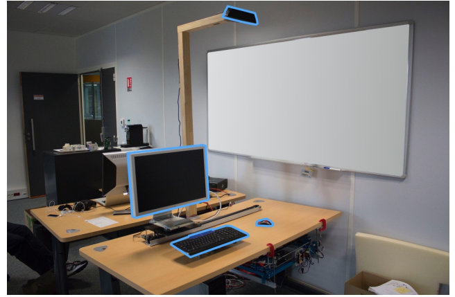
Figure 2. Living Desktop setup consisting of a mouse, keyboard and monitor as well as a depth camera to track their position on the desk.
