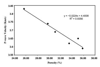
Figure 4. P-wave velocity versus porosity for saturated samples.
