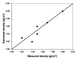
Figure 10. Estimated density and measured density from P-wave velocity for saturated samples.
