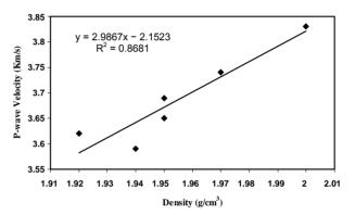
Figure 6. P-wave velocity versus density for saturated samples.
