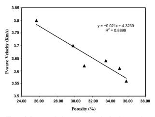
Figure 3. P-wave velocity versus porosity for dry samples.
