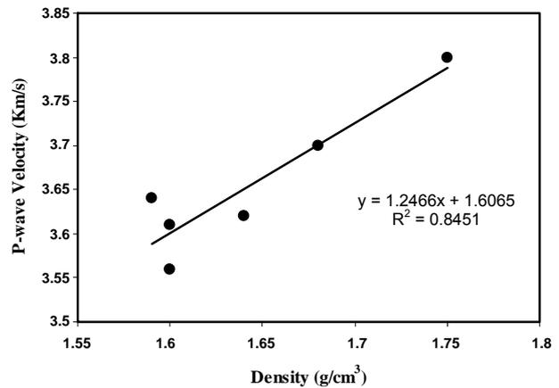
**Figure 5.** P-wave velocity versus density for dry samples.
