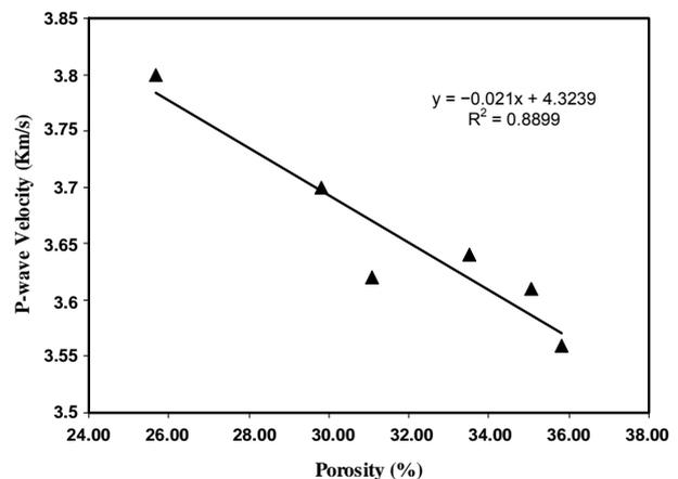
**Figure 3. P-wave velocity versus porosity for dry samples.**
