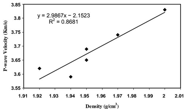
**Figure 6.** P-wave velocity versus density for saturated samples.
