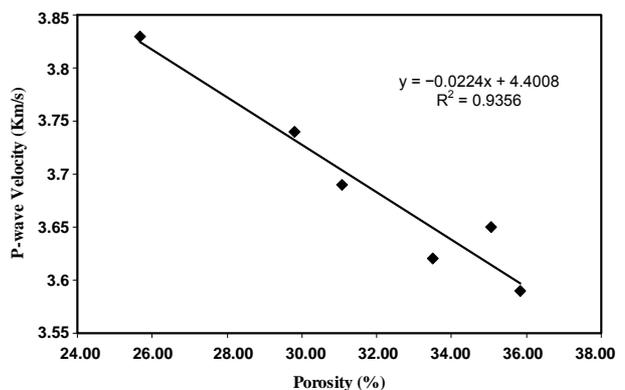
**Figure 4. P-wave velocity versus porosity for saturated samples.**
