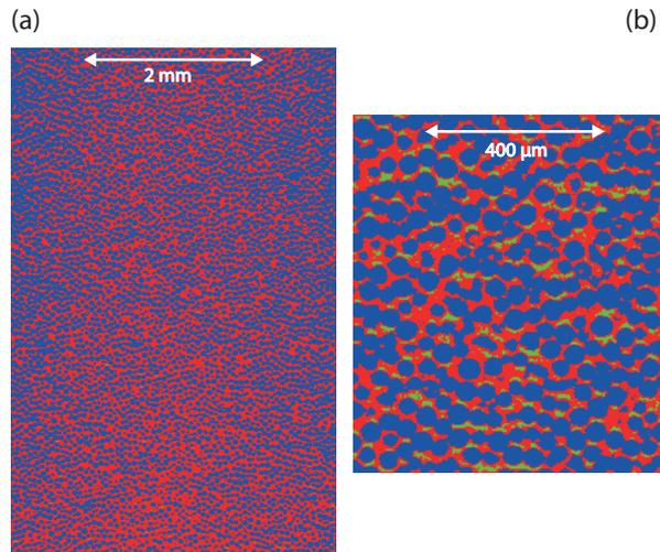
**Fig. 10** Thresholded tomographic slice through a specimen of polyacrylate/glass beads composites filled with small particles only at 0.15 macroscopic strain. The loading direction is vertical. (a) Image obtained with the tomograph settings presented in section 2.2 and (b) enlarged view.
