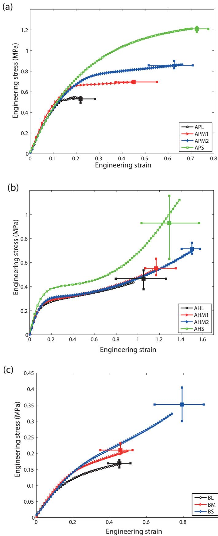
**Fig. 5** Uniaxial tension stress-strain behavior of propellants containing different matrices and particles. (a) Matrix A filled with ammonium perchlorate, (b) matrix A filled with HMX, and (c) matrix B with HMX.
