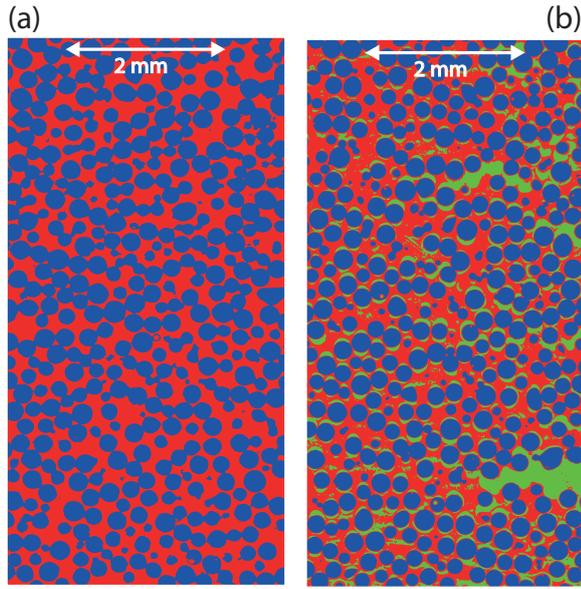
**Fig. 9** Thresholded tomographic slices through specimens of polyacrylate/glass beads composite filled with large particles only at: a) 0 macroscopic strain and b) 15% macroscopic strain. The loading direction is vertical.
