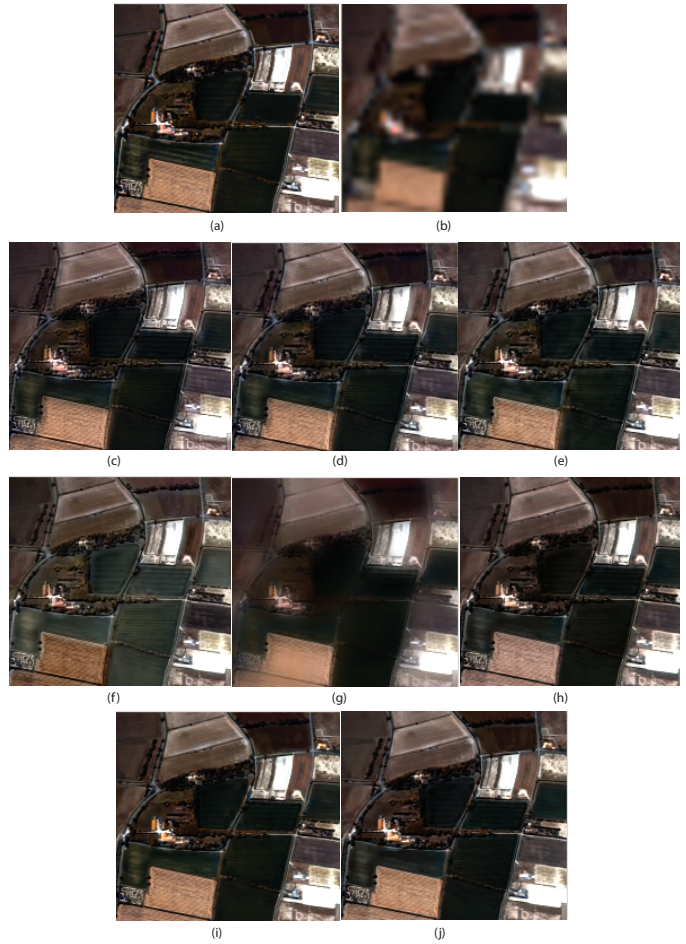
Fig. 6. Details of original and fused Camargue dataset HS image in the visible domain. (a) reference image, (b) interpolated HS image, (c) SFIM, (d) MTF-GLP-HPM, (e) GSA, (f) PCA, (g) GFPCA, (h) CNMF, (i) Bayesian Sparse, (j) HySure
