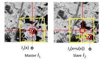
Figure 1. Definition of variables used in our optical-flow algorithm: To register the slave image  $I_2$  to the master image  $I_1$ , we model the displacements between both images  $\mathbf{u}(\mathbf{x})$  for each pixel x in the master image. Corresponding pixels  $I_1(\mathbf{x})$  and  $I_2(\mathbf{x} + \mathbf{u}(\mathbf{x}))$  are supposed to be close with respect to a similarity measure.
