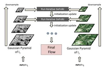
Figure 3. To enable the recovery of large displacements, a multi scale strategy is employed: After the generation of image pyramids for master and slave image, the optical flow is computed from coarse to fine, by minimizing the cost function (eq 3).
