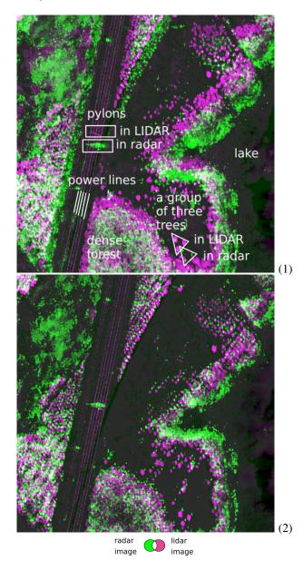
Figure 8. Result of coregistation for DSM LIDAR data on a 1,000 x 1,000 pixel SAR image sample over Remningstorp forest (Sweden) (1) after coregistration by geocoding using SRTM, (2) after coregistration by geocoding using GSD50+ DEM
