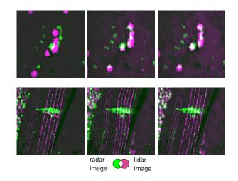
Figure 11. Result of coregistation for LIDAR data and SAR image over Remningstorp forest (Sweden) for two 100 x 100 pixel extracts (1) after coregistration by geocoding (2) after coregistration by the baseline algorithm based on Mutual Information, (3) after coregistration by **GeFolki**
