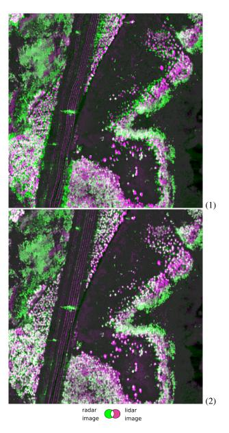
Figure 9. Result of coregistation for DSM LIDAR data on a 1,000 x 1,000 pixel SAR image over Remningstorp forest (Sweden) (1) after coregistration by an algorithm based on Mutual Information, (2) after coregistration by **GeFolki**
