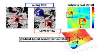
Figure 2. General minimization scheme by an iterative method. On the left: master image with a local window under consideration. In the middle: Two candidate regions in the slave image. The correct match is highlighted in red, another window with high similarity in blue. On the right: The matching cost is in general a non-convex function. Below: When started within sufficient proximity to the true minimum, gradient descent based optimization can recover the correct solution.
