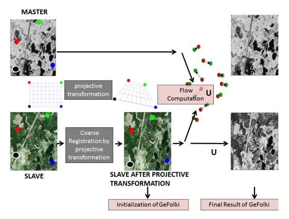
Figure 7. Coregistration scheme by optical flow calculation: first a coarse coregistration is performed by warping the slave image on the master image trough a projective transformation based on the manual selection of four tie-points. This first step constitutes the initialization of **GeFolki**. Then, **GeFolki** computes the flow for this couple of images, and the final slave image is resampled accordingly.
