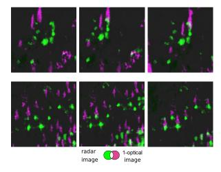
Figure 14. Result of coregistation for optical data and SAR image over Remningstorp forest (Sweden) for two 100 x 100 pixel samples (1) after coregistration by geocoding (2) after coregistration by an algorithm based on Mutual Information, (3) after coregistration by **GeFolki**
