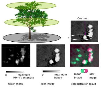
Figure 10. Effects of geometry on the signature of a tree in the scene for polarimetric radar images and for LIDAR image. Example on a very small 30 x 40 pixel extract of the different products containing four trees: polarimetric SAR image on the left, DSM LIDAR image on the middle, and superposition after our best coregistred product on the right
