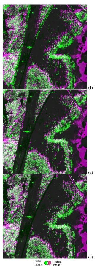
Figure 13. Result of coregistation of an optical image on a 1,000 x 1,000 pixel SAR image over Remningstorp forest (Sweden) (1) after coregistration by geocoding (2) after baseline coregistration based on Mutual Information, (3) after coregistration by **GeFolki**
