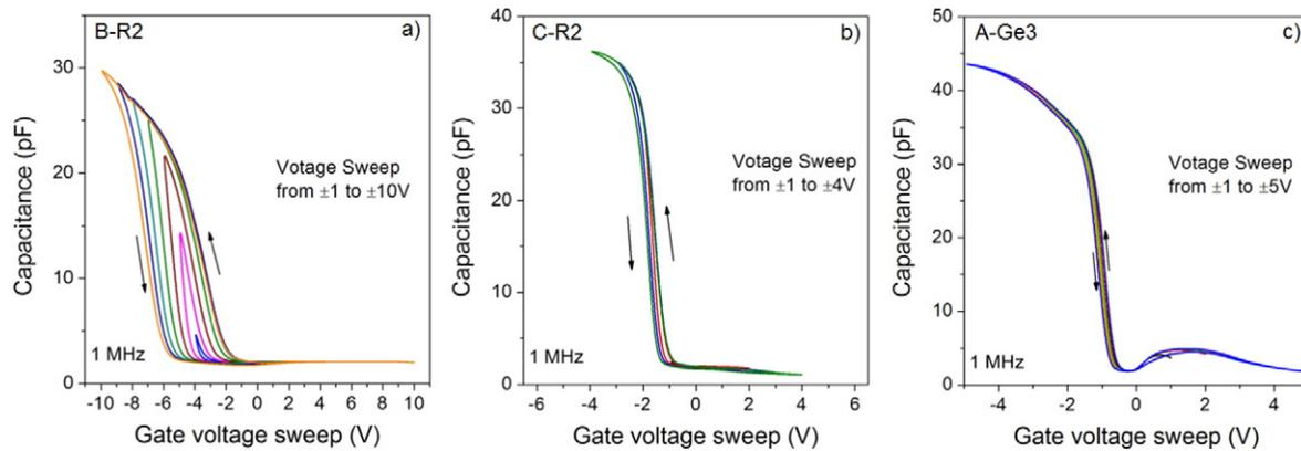
Fig. 5. The C–V data for the samples C-R2 (a), B-R2 (b) and A-Ge3 (c). The samples were annealed at 800 °C for 30 min in N<sub>2</sub> flow. The measurements were performed in darkness.
