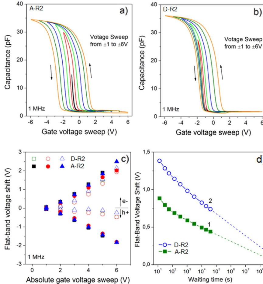
**Fig. 4.** The C-V data for the samples A-R2 (a) and D-R2 (b). (c) Extracted flat-band voltage shift as a function of the gate voltage sweep for A-R2 and D-R2. (d) Charge retention characteristics at room temperature for the A-R2 (1) and D-R2 (2) samples after application of a gate voltage of +6 V for 10 s. Extrapolation curves for a 10-year waiting time are also reported. The samples were annealed at 800 °C for 30 min in N<sub>2</sub> flow. The measurements were performed in darkness.
