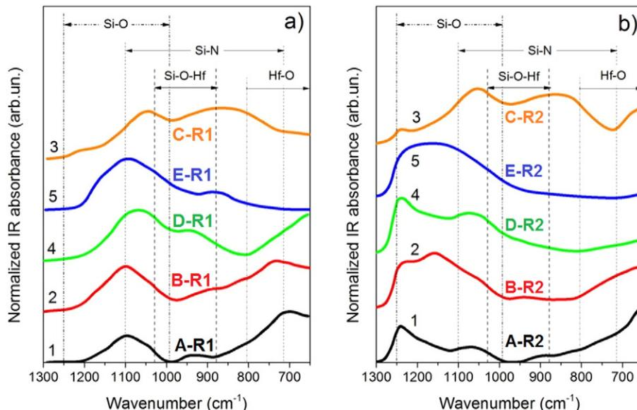
Fig. 1. Normalized ATR–FTIR spectra of the samples A (1), B (2), C (3), D (4) and E (5): a) as-deposited (marked with R1) and b) annealed at 800 °C for 30 s in N<sub>2</sub> flow (marked with R2).
