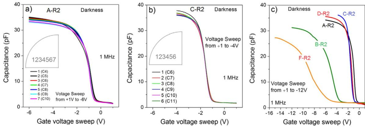
**Fig. 3.** The single sweep C-V data for samples A-R2 (a) and C-R2 (b), demonstrated the uniformity of electrical properties. c) The comparison of single sweep C-V curves for different structures mentioned in the figure. All measurements were performed in darkness. The samples were annealed at 800 °C for 30 min in N<sub>2</sub> flow.
