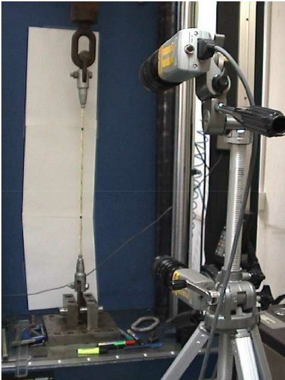
Fig. 10. Test on assembled yarn sample on 200 kN test machine, showing sample and two digital cameras to measure strain.
