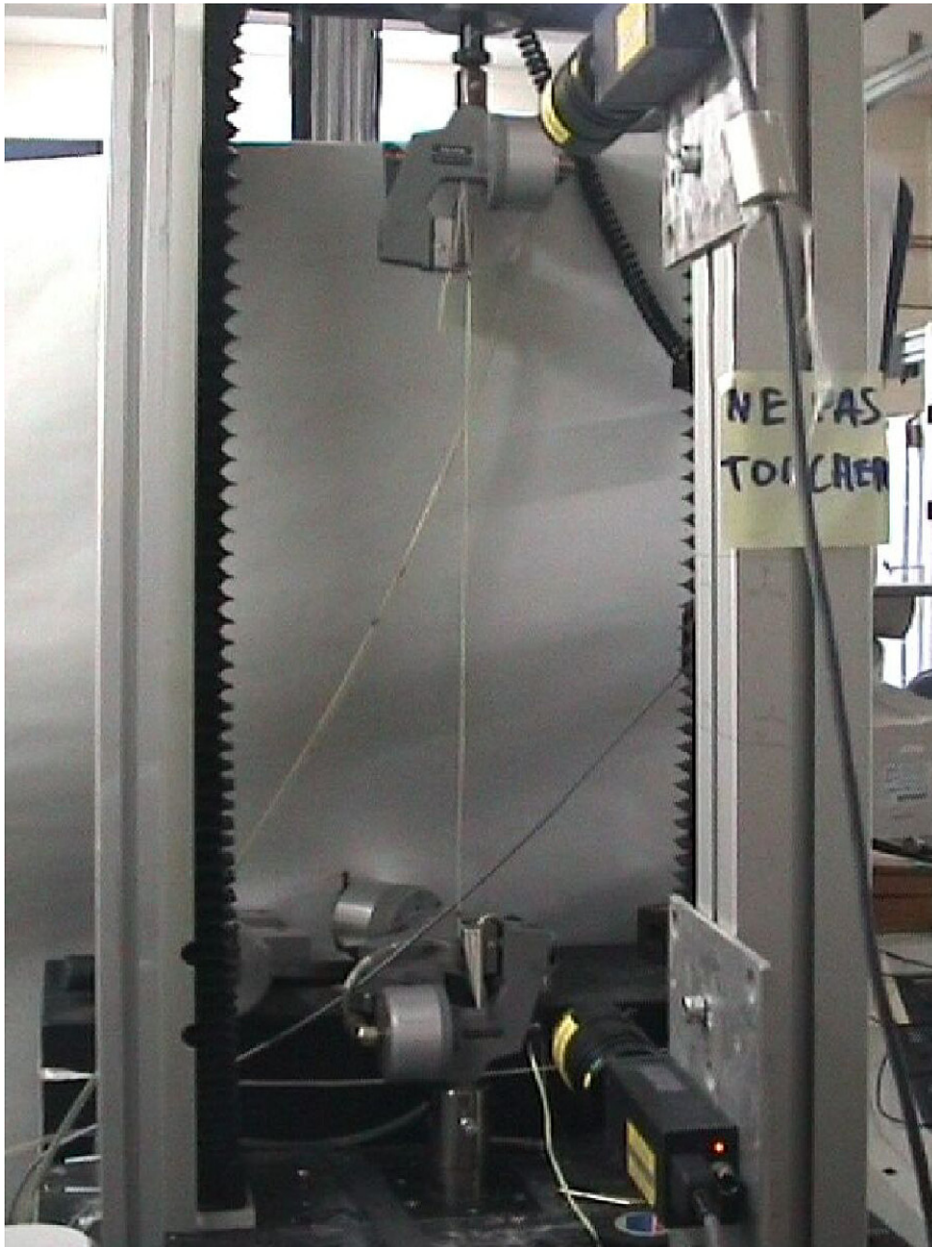
Fig. 8. Testing of yarns on 10 kN test machine, two digital cameras to measure strain.
