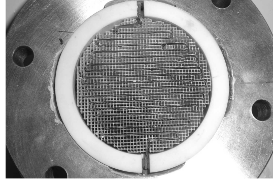
Figure 4: Hot heat exchanger inserted in the insulating ceramic ring.
