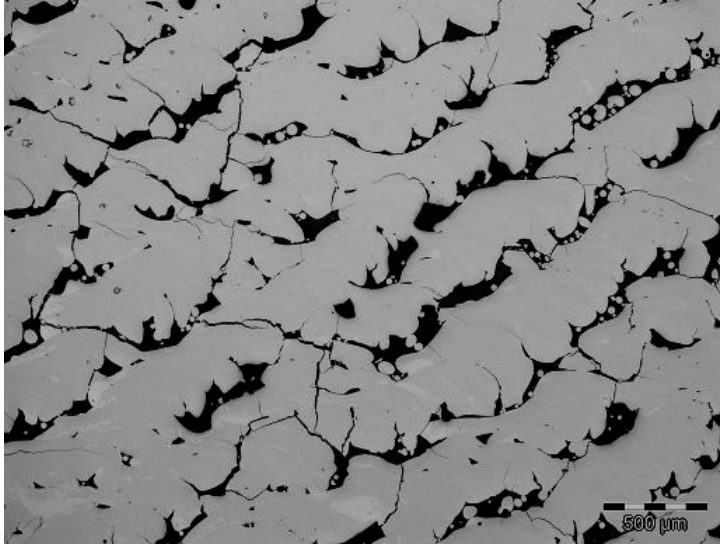
Figure 2: Optical microscopy of XY surface layers using the following parameters: power 50 W, speed 60 mm/s, distance between two laser lines 200 μm
