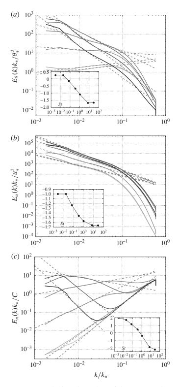
FIGURE 13. Temperature (a), velocity (b) and particle concentration (c) spectra, for the various Stokes numbers (St = 0.003, 0.019, 0.074, 0.352, 1.064, 7.343 and 29.36, from light grey to black respectively) at  $\gamma = 570$ , C = 0.19. Comparison with the power law obtained by fit of the DNS in dashed lines. Insert: exponent of the power law as a function of the Stokes number.
