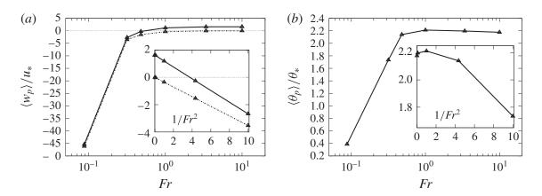
FIGURE 23. Evolution with the Froude number of (a) the mean vertical particle velocity and comparison with the Stokes terminal velocity  $u_{\tau} = \tau_p g$  (dashed lines) and (b) the mean particle temperature, for  $\gamma = 80$  and St = 0.3 C = 0.35, normalized by the critical values  $u_*^2$  and  $\theta_*$ . Inserts: evolution with  $Fr^{-2}$  in linear scales.
