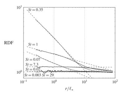
FIGURE 6. Radial distribution function (RDF) for the various Stokes numbers (St = 0.003, 0.019, 0.074, 0.352, 1.064, 7.343 and 29.36, from light grey to black respectively) at  $\gamma = 570$ , C = 0.19. Comparison with the power law obtained by fit of the DNS in dashed lines.
