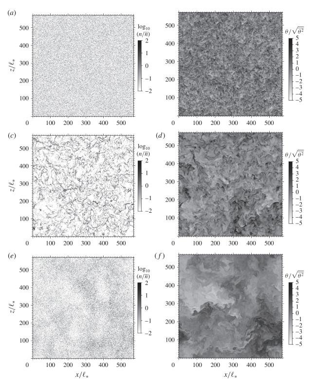
FIGURE 1. Visualization in a x-z plane: (a,c,e) of the logarithm of the particle concentration field (as computed by (3.1)) normalized by the mean concentration  $n/\overline{n}$ , and (b,d,f) the fluid temperature fluctuations normalized by its standard deviation  $\theta/\overline{\theta^2}^{1/2}$ . For  $\gamma = 570$  and C = 0.19, at three Stokes numbers: St = 0.003 (a,b), St = 0.352 (c,d) and St = 7.343 (e,f).
