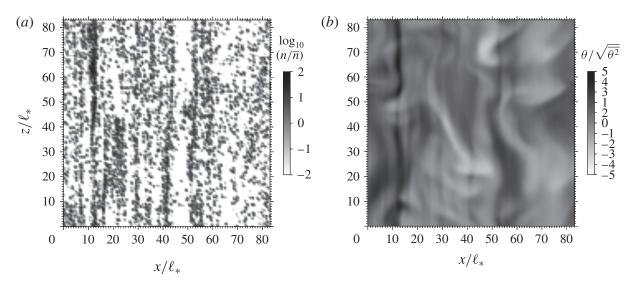
FIGURE 22. Snapshots in a x-z plane: (a) of the logarithm of the particle concentration field (as computed by (3.1)) normalized by the mean concentration  $n/\overline{n}$ , and (b) the fluid temperature fluctuations normalized by its standard deviation  $\theta/\overline{\theta^2}^{1/2}$ . For  $\gamma = 80$  and C = 0.35, St = 0.352 and Fr = 0.09.
