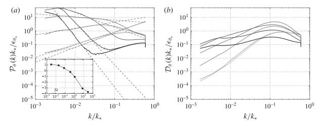
FIGURE 14. Temperature forcing (a) and temperature dissipation (b) spectra defined in (4.25), for the different Stokes numbers (St = 0.003, 0.019, 0.074, 0.352, 1.064, 7.343 and 29.36, from light grey to black respectively) at  $\gamma = 570$ , C = 0.19. Comparison with the power law obtained by fit of the DNS in dashed lines. Insert: exponent of the power law as a function of the Stokes number.
