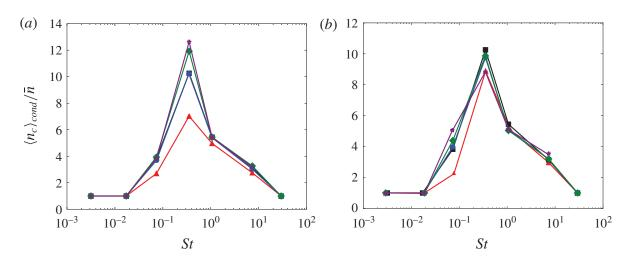
FIGURE 10. (Colour online) Mean particle concentration in large clusters as a function of the Stokes number. (a) For  $\gamma=83$  and C=0.035 (red triangles), 0.19 (black squares), 0.35 (blue circles), 1.82 (green squares), 8.77 (purple stars); (b) for C=0.19 and  $\gamma=48$  (red triangles), 83 (black squares), 190 (blue circles), 330 (green squares) and 570 (purple stars).
