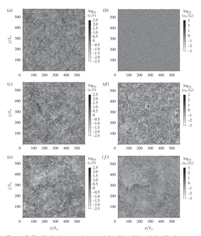
FIGURE 2. Visualization in a x–z plane: (a,c,e) logarithm of the turbulent kinetic energy dissipation rate normalized by its mean value  $\log_{10}(\varepsilon/\overline{\varepsilon})$  and (b,d,f) logarithm of the temperature fluctuation dissipation rate normalized by its mean value  $\log_{10}(\varepsilon_{\theta}/\overline{\varepsilon_{\theta}})$ . For  $\gamma=570$  and C=0.19, at three Stokes numbers: St=0.003 (a,b), St=0.352 (c,d) and St=7.343 (e,f).
