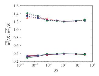
FIGURE 19. (Colour online) Evolution with the Stokes number of the variance of the horizontal (continuous lines) and vertical (dashed lines) velocity components both normalized by the mean turbulent kinetic energy K. For  $\gamma = 83$  and C = 0.035 (red triangles), 0.19 (black squares), 0.35 (blue circles), 1.82 (green squares), 8.77 (purple stars).
