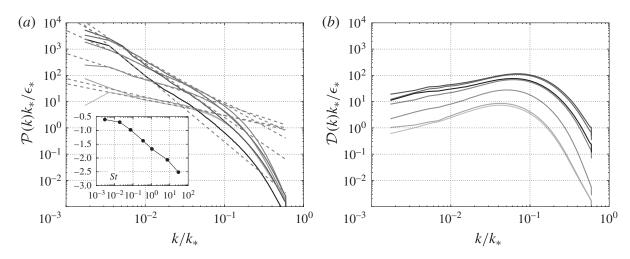
FIGURE 15. Forcing (a) and dissipation (b) spectra of the turbulent kinetic energy as defined in (4.26) for the different Stokes numbers (St = 0.003, 0.019, 0.074, 0.352, 1.064, 7.343 and 29.36, from light grey to black respectively) at  $\gamma = 570$ , C = 0.19. Comparison with the power law obtained by fit of the DNS in dashed lines. Insert: exponent of the power law as a function of the Stokes number.
