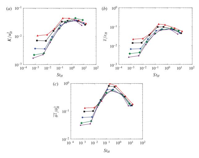
FIGURE 12. (Colour online) Turbulent kinetic energy (a), the dissipation rate of turbulent kinetic energy (b), the fluid temperature variance (c) normalized respectively by  $u_H^2$ ,  $\varepsilon_H$  and  $\theta_H$  plot against  $St_H$  in log-log scales. For C=0.19 and  $\gamma=48$  (red triangles), 83 (black squares), 190 (blue circles), 330 (green squares) and 570 (purple stars).
