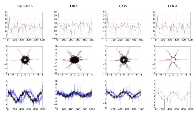
Fig. 7. Centroids obtained from a set of height noisy instances  $\{(x_k, y_k)\}_{k=1...8}$  for Euclidean, DBA, CTW and TEKA averaging methods. The log power spectra in dB (top), the 2D shape (center) and x,y waveforms (bottom) are shown.
