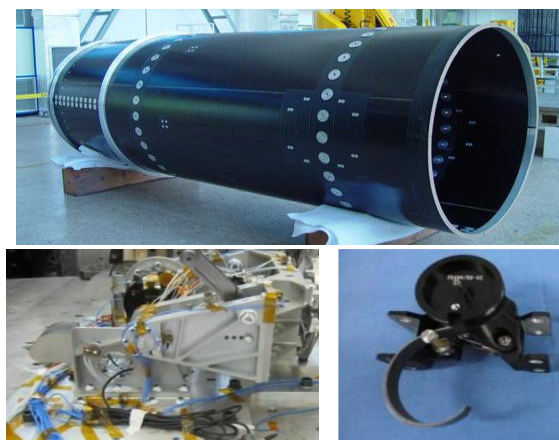
Figure 8: Central cylinder with flight heritage.
