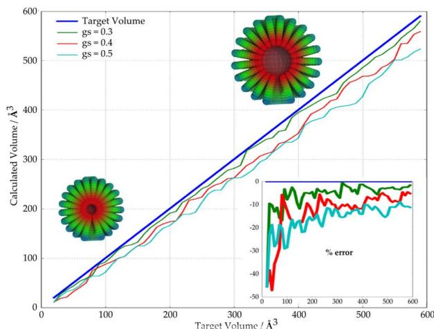
**Figure 23:** Example of volume measurement error assessment based on a sphere cavity trajectory of precisely controlled volume. The true sphere volume increases regularly (blue line). Three program settings are compared with percentual error indicated as inset. The smallest and largest spherical cavities are depicted. Data kindly provided by Dr. Benoist Laurent.
