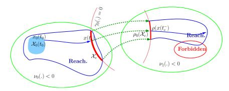
FIGURE 1. Set reachable in finite time by system (2-4).
