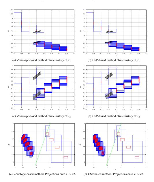
FIGURE 5. Reachable set computed for (29). Zonotope-based method, CPU times=0.16*s*. CSP-based method, CPU times=0.20*s*.
