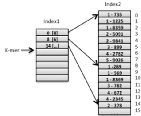
Figure 2: Index1 provides for all possible k-mer its number of occurrences and an entry in Index2. Index2 is a list of coordinates specifying the chromosome number and a position.
