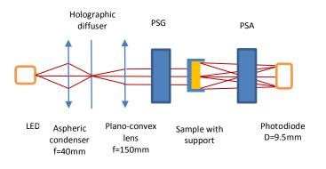
Fig. 1. Schematic presentation of the Mueller matrix polarimeter
