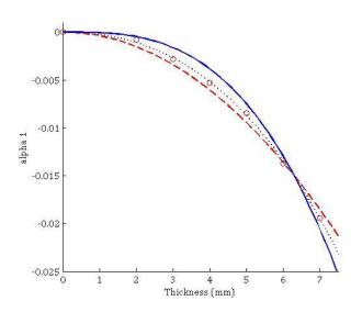
Fig. 10. Evolution of the logarithmic depolarizations  $\alpha_1$  with *z* the thickness of medium traveled by light for a dilutions d = 0.13 of milk. o are experimental values. Light is collected by a lens (focal length f = 140mm). Solid line and dashed line are respectively the best cubic and parabolic fit. The dotted line is derived from Eq. (12).
