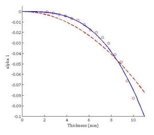
Fig. 9. Evolution of the logarithmic depolarizations  $\alpha_1$  with z the thickness of medium traveled by light for a dilutions d = 0.13 of milk. o are experimental values measured with the measurement setup depicted Fig. 1. Solid line and dashed line are respectively the best cubic and parabolic fit.
