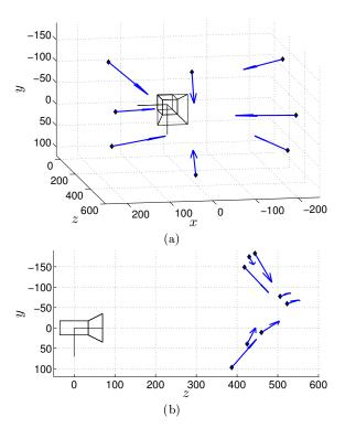
Fig. 5 Two views of a schematic representation of the experimental setup of Fig. 2-a. The camera center is located in (0,0,0). A black marker characterizes the location  $\mathbf{x}_s$  of each LED (unit mm), the orientation of a blue arrow its principal direction  $\mathbf{n}_s$ , and the length of this arrow its intensity  $\Phi_0$  (up to a common factor).
