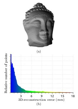
Fig. 12 (a) 3D-reconstruction obtained with Algorithm 2, using the result from Fig. 7-a as initial guess. (b) Histogram of point-to-point distances between this 3D-shape and the ground truth (cf. Fig. 7-c). The median value is 1.2 mm.
