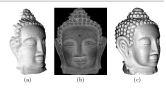
Fig. 7 (a) 3D-reconstruction and (b) albedo obtained with Algorithm 1. (c) Ground truth 3D-shape obtained by laser scanning. Photometric stereo not only provides a 3D-shape qualitatively similar to the laser scan, but also provides the albedo.
