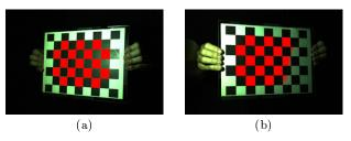
Fig. 4 Two out of the q poses of the Lambertian planar calibration pattern used for the photometric calibration of the LEDs. The parts of the white cells which are used for estimating the LEDs principal directions and intensities are highlighted in red.
