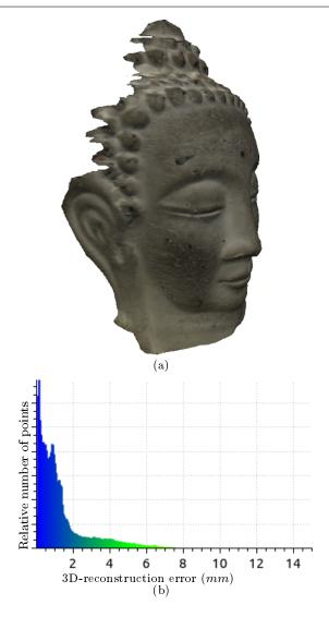
Fig. 17 (a) 3D-model estimated from the m=8 images of Fig. 2, which are RGB images. (b) Histogram of the distances between this 3D-shape and the ground truth (cf. Fig. 7-c). Using RGB images improves the result, in comparison with the experiment of Fig. 15: the median of the point-to-point distances to the ground truth is now equal to  $0.85 \ mm$ .
