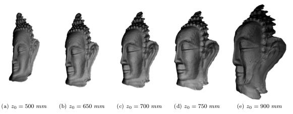
Fig. 10 3D-reconstructions after 10 iterations of the ADMM scheme, taking as initial guess different fronto-parallel planes  $z \equiv z_0$ . The median of the distances to ground truth is, from left to right: 3.05 mm, 2.88 mm, 1.68 mm, 2.08 mm and 5.86 mm. When the initial guess is too close to the camera, the 3D-reconstruction is flattened, while the scale is overestimated when starting too far away from the camera (although this yields a lower energy, see Fig. 11).
