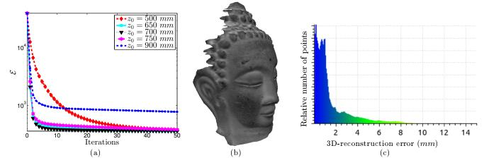
Fig. 15 Same as Fig. 13, but using Cauchy's robust M-estimator and explicit self-shadows handling. Despite the non-convexity of the estimator, convergence is similar to that obtained in the previous experiment. However, the median value of the 3D-reconstruction error is now 0.91 mm, which is to be compared with the previous value 1.2 mm (cf. Fig. 13).
