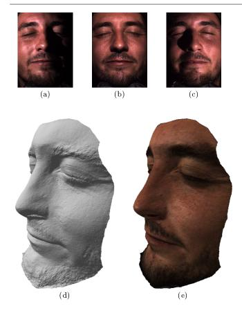
Fig. 18 (a-b-c) Three RGB images (out of m=8) of a face captured by our setup. (d) Estimated 3D-shape. (e) Colored 3D-model. Since their estimation is relative to the Lambertian planar calibration pattern, the colored albedos of the 3D-model may appear different from the colors of the images.
