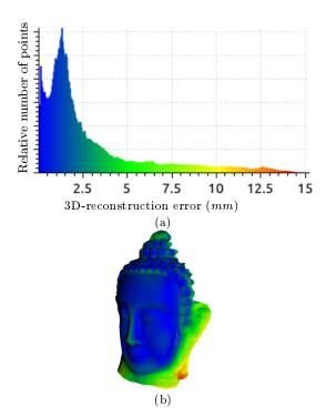
Fig. 8 (a) Histogram of point-to-point distances between the alternating 3D-reconstruction and the ground truth (cf. Fig. 7). The median value is 1.3 mm. (b) Spatial distribution of these distances. The histogram peak is not located in zero. As we will see in Section 3.2, this bias can be avoided by resorting to a differential approach based on PDEs.
