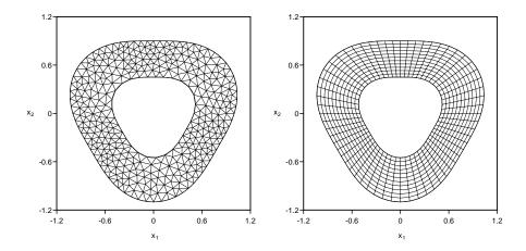
Figure 9: Coarse uniform triangular Delaunay mesh (left panel) and uniform quadrilateral mesh (right panel) prescribed for the rose-shaped domain.
