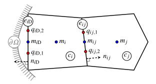
Figure 1: Mesh notation with edge and cell reference points (blue dots), Gauss points (red dots associated to a two-point quadrature rule), and unit normal vectors (dashed lines).
