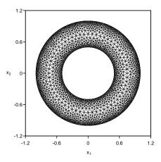
Figure 6: Coarse non-uniform triangular Delaunay mesh prescribed for the annulus domain for the high Péclet number test case.
