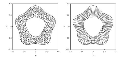
Figure 11: Coarse uniform triangular Delaunay mesh (left panel) and uniform quadrilateral mesh (right panel) prescribed for the rose-shaped domain.
