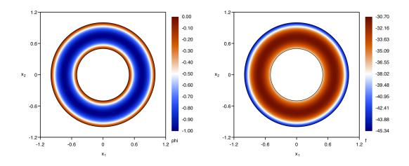
Figure 3: Manufactured solution (left panel) and source term (right panel) for the low Péclet number test case.
