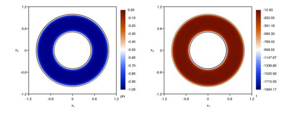
Figure 5: Manufactured solution (left panel) and source term (right panel) for the high Péclet number test case.
