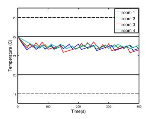
Figure 7: Example 5.3: Simulation from the initial condition (22, 22, 22, 22). The objective set R is in plain black and the safety set S is in dotted black.
