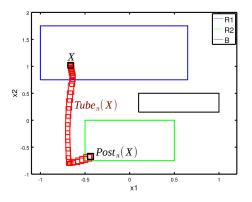
Figure 2: Illustration of functions  $Post_{\pi}(X)$  and  $Tube_{\pi}(X)$  from the Example 5.2, for the initial box  $X = x1 \times x2 = [-0.69, -0.64] \times [1, 1.06]$ , with a pattern  $\pi = (1, 3, 0)$ .
