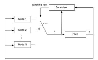
Figure 1: Sampled switched systems (with u the input and y the state of the system)
