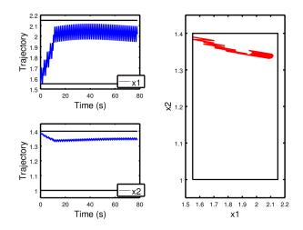
Figure 4: Example 5.1: Simulation from the initial condition (1.55, 1.4). The box R is in plain black. The trajectory is plotted within time for the two state variables on the left, and in the state space plane on the right.
