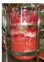
Fig. 2 : 1.5 L fermentor allowing fungal growth and pigments production
