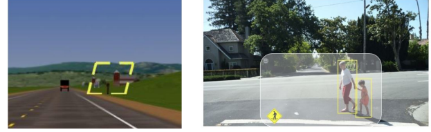
(a) Example of a pedestrian highlighting [24] (b) The proposed visual cues for Pedestrian Collision Warning Systems.
