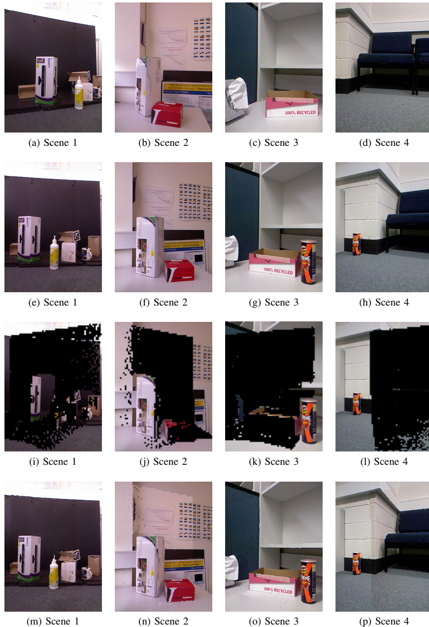
Fig. 6: A demonstration of the scheme over four sets of images: First and second rows show the images captured by sensors a , and b respectively. In the third row, image blocks transmitted by sensor b are shown (here black regions denote the image blocks that are not transmitted). The fourth row shows the reconstructed images at the receiver side using the data sent by sensor b .
