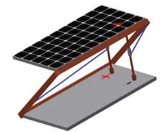
Fig. 2. Sketch of one coil connected to its 2 corresponding solar cells. The other coil is the same, but rotated by  $90^{\circ}$  around the *z*-axis.
