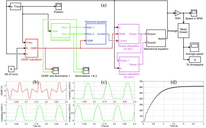
Fig. 4. (a) Simulink diagram of the whole motor. (b) Illustration of the counter-electromotive force on "coil 1" (up) with the corresponding illumination "Illum. 1" of one solar cell. (c) Illumination of two solar cells on both sides of the rotor vs. time. (d) Example of temporal evolution of the speed of the rotor.
