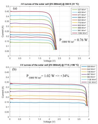
Fig. 5. I - V curves of the solar cell 2 V – 380 mA for different positions from the light source, i.e. for different irradiances: (a) at ambient air temperature 304 K and (b) in liquid nitrogen at 77 K. The delivered power by the solar cell has increased of +34% for the same irradiance of 1000 W/m<sup>2</sup>.
