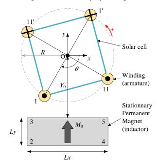
Fig. 1. Illustration of the machine with the labels used to identify the dimensions. The inductor, a Permanent Magnet (PM) delimited by its corners  $\{2, 3, 4, 5\}$ . The armature is composed of 2 coils, sketched as 4 wires labeled  $\{1, 1', 11, 11'\}$ .
