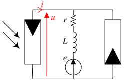
Fig. 3. Electric diagram of the armature with an illuminated solar cell on the left.
